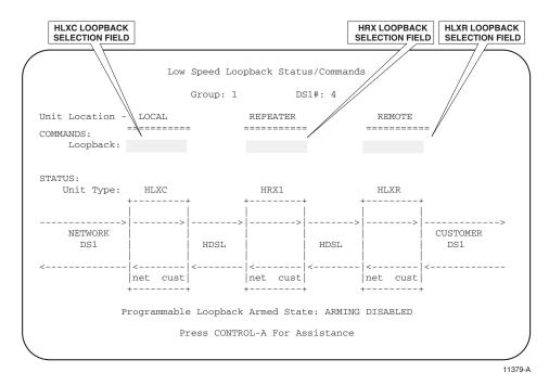
Figure 541-4. Low Speed Loopback Status/Commands Screen
